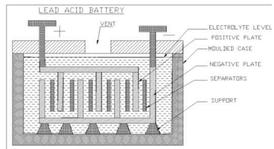
**Fig. 3 Lead Acid Battery**
