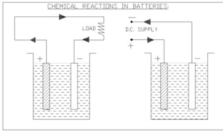
**Fig. 4 Chemical Reactions in Batteries.**
