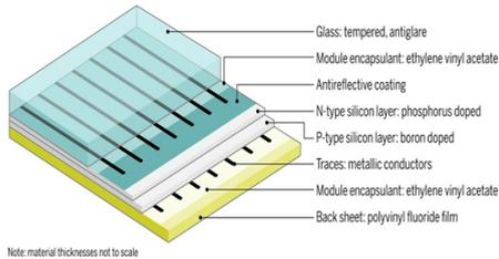
(Fig. 1 Components of a typical silicon solar cell.)
