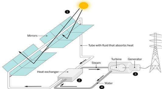
(Fig. 4 Schematic of a typical 1D concentrating solar thermal system.)
