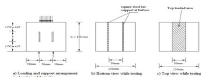
**Plate 2.1: Details of DCN specimen geometry**
