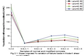
Fig 2.1 Super imposed variation of failure loads in Mode-II shear wr to LVAC
