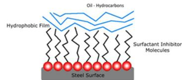
Fig 3: Mechanism of a conventional corrosion inhibitor
